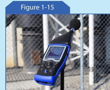
The XL2-TA from NTI Audio offers not only sound level metering but also advanced analysis features, such as RTA, RT60/RMS level, distortion measurement, oscilloscope function and more.
