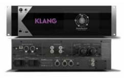
audio setup and monitoring meters; the headphone amp delivers studio-grade fidelity; the front PoE network port can power a KLANG:controller or KLANG:quelle; and dual redundant power supplies offer maximum reliability.
