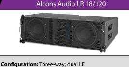
LF: (2) 8" woofers MF: 6.5" cone midrange HF: 7" ribbon driver Frequency Response: 70 Hz to 20 k Hz (±3 dB) Dispersion (HxV): 120° x 10°
