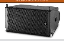
LF: (2) 12" neodymium woofers MF/HF: (2) coaxial 6" planar-wave drivers **Frequency Response:** 50Hz to 22kHz **Horizontal Dispersion:** Variable 90/100/110° **Size:** 26.5 x 14.7 x 22.5"
