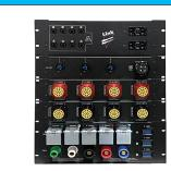
Input: 200A main input with Cam-Lok in and pass-thru Outputs: Digital multi-function power meter-network output: (4) sets of LKS Data 120/208V outputs: shared 2-pole breakers; (4) L21-30 outs; Edison duplex outlets Enclosure Type: Freestanding 19" rack mount
