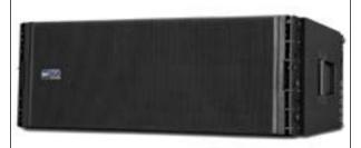
**LF:** (2) 12" neodymium woofers **MF:** 10" cone neodymium mid **HF:** (3) 1.5" exit neodymium drivers **Frequency Response:** 50 Hz to 20k Hz
