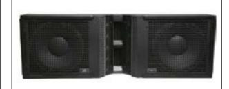
**LF:** (2) 12" neodymium Black Widow woofers **MF:** (10) 2.5-inch cone neodymium mids **HF:** (4) 4.75" planar ribbon tweeters **Frequency Response:** 70 Hz to 20k Hz
