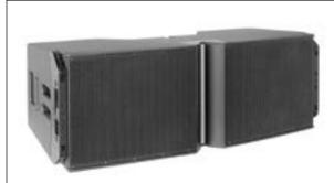
**LF:** (2) 12" neodymium woofers MF: (4) 6.5" cone neodymium mids HF: 14" RBN pro ribbon driver Frequency Response: 51 Hz to 20k Hz Horizontal dispersion: 80° **Size (HxWxD):** 15.8 x 43.4 x 21.1"
