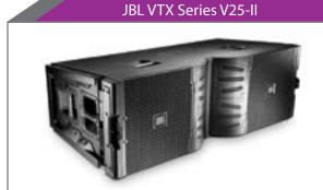
**LF:** (2) 15" 2267H neodymium woofers MF: (4) 8" 2169H cone neodymium mids **HF:** (3) 2430K D2 Dual Drivers Frequency Response: 35 Hz to 18k Hz
