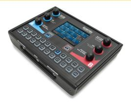
A Livemix system is based on a MX-16 or MX-32 central mixer/distributor (with analog or Dante inputs) and any number of CS-DUO personal mixers, each one of which offers two separate mixes, so eight performers, only requires four CS-DUO units. Features include up to 24 channels with button, knob and touchscreen control; EQ, HPF and dynamics on every channel; and a dedicated "me" knob.
