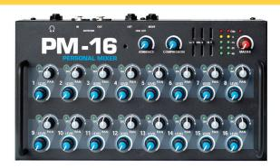
Up to 16 analog channels enter a PM-16 input module, which outputs Cat-5 to a DM-8 distribution module that sends power and signals to up to eight PM-16 personal mixers, each with ambient mic, 16 gain and pan pots, graphic EQ and compressor. More DM-8's can cascade for adding more PM-16's to form larger systems.
