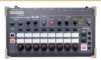
The M-48 connects via REAC (Roland Ethernet Audio Communication) protocol to a Roland digital console or S-4000S/S1608 digital snake system or any MADI-equipped digital mixer (using the S-MADI REAC-MADI Bridge). The system adds remote individual monitor control of up to 40 audio channels via 16 stereo groups, with volume, pan, 3-band EQ and built-in reverb per group and an output (ear protection) limiter is standard. All M-48 mixers link to the system using Cat-5 cabling.
