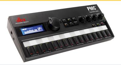
PMC offers 16 channels of audio with EQ, pan, Stereo Width control and effects, including Lexicon reverbs and dbx PeakStopPlus limiting. Performers can mix in real-time and save 16 user-preset mixes. PMC uses a BLU link audio bus from a dbx TR1616 or any BSS London system, supporting up to 60 PMC16 mixers on a single BLU Link Ring at up to 96 kHz. USB, DSC and Ethernet ports allow future updates.
