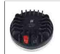
MAGNET **IMPEDANCE** Neodymium 8 ohm DIAPHRAGM **VOICE COIL** POWER RATING WEIGHT 100 watts 6.8 pounds FREQUENCY RESPONSE 500 Hz to 18k Hz Four M6 holes on 4-inch SENSITIVITY 112 dB, 1w/1m
