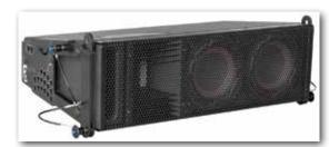
Configuration: Two-way; dual LF **LF:** (2) Neodymium 6.5" HF: 4" Alcons RBN401 ribbon driver Frequency Response: 74 Hz to 20kHz Dispersion (HxV): 90° x 15°
