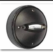
Magnet: Ferrite Diaphragm: PETB film Power Rating: 80 Watts Frequency Response: 800 Hz to 18 kHz Impedance: 8 ohms Voice Coil: 1.75" **Crossover Frequency:** >1.2 kHz Weight: 6 pounds
