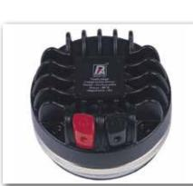
Magnet: Neodymium **Diaphragm:** Titanium Power Rating: 80 Watts Frequency Response: 1 kHz to 20 kHz Sensitivity: 110 dB SPL, 1W/1m Impedance: 8 ohms Voice Coil: 1.75" **Crossover Frequency:** >1.5 kHz Weight: 4.2 pounds
