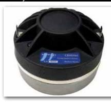
Magnet: Neodymium Diaphragm: Aluminum Power Rating: 70 Watts Frequency Response: 700 Hz to 19k Hz Sensitivity: 111 dB SPL, 1W/1m Impedance: 8 ohms Voice Coil: 1.75" Crossover Frequency: >1.2 kHz Weight: 2.7 pounds Mount: 2-hole or 3-hole bolt-on
