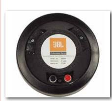
Magnet: Ferrite Diaphragm: Titanium **Power Rating:** 70 Watts Frequency Response: 800 Hz to 20 kHz **Sensitivity:** 110 dB SPL, 1W/1m Impedance: 8 ohms (2426J 16-ohm also
