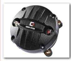
**Diaphragm:** PETP film Power Rating: 75 Watts Frequency Response: 1.2 kHz to 20 kHz Sensitivity: 110 dB SPL, 1W/1m Impedance: 8 ohms Voice Coil: 1.75" Crossover Frequency: >2.2 kHz Weight: 1.4 pounds **Mount:** 4-hole bolt-on (M6 thread)
