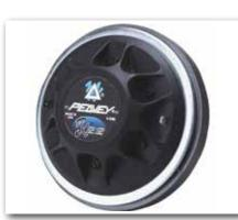
Magnet: Ferrite **Diaphragm:** Titanium Power Rating: 70 Watts Frequency Response: 500 Hz to 20 kHz Sensitivity: 111 dB SPL, 1W/1m Impedance: 8 ohms Voice Coil: 2" Crossover Frequency: >1.2 kHz
