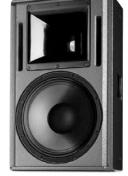
LF: 12" woofer HF: 1" exit comp. driver Response: 48Hz to 20kHz **Dispersion:** 80 x 50° (rotatable) Size: 26.2x15.2x15' Weight: 45.4 pounds Rigging: (6) M10; pole cup
