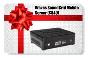
It's tiny, but packs a powerful punch, with an onboard Intel Core i5 processor and 4 GB of RAM that's ideal for boosting your plug-in processing power. Latency is a low 0.8 ms at 44.1k to 96k Hz. Use with any SoundGrid audio interface (including DiGiGrid I/O's) for real-time processing for live-mixing/recording with plug-ins. The downside? It doesn't ship until early 2019, but some things are worth waiting for.
