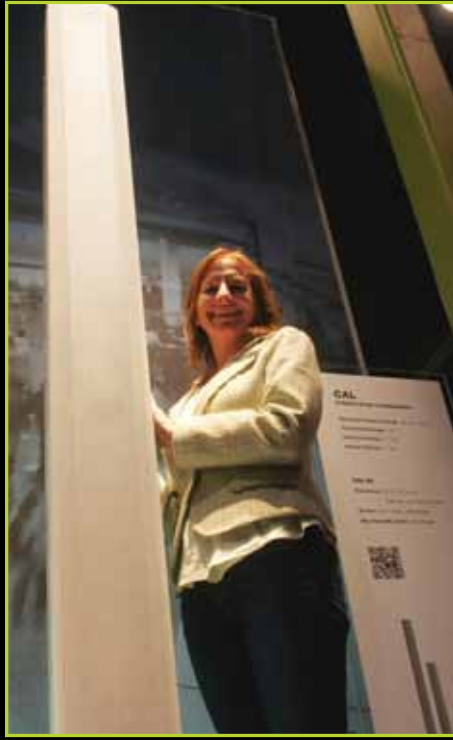
Meyer Sound's Rachel Archibald with CAL , their new self-powered two-way steerable column array loudspeaker that employs 4-inch woofers and 20-mm tweeters. CAL's vertical beam can be angled up or down 30 degrees and can be opened vertically from five to 60 degrees.
