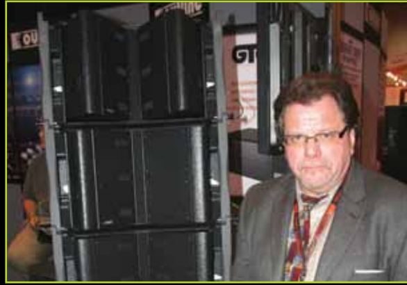
Outline's U.S. VP and MD Tom Bensen with their Mini-COM.P.A.S.S. iMode adjustable compact line array. Each module weighs only 53 pounds, employing dual 1.75-inch compression drivers and four five-inch cones. Horizontal coverage can be set between 60 and 150 degrees in 15 degree steps to fine-tune coverage.
