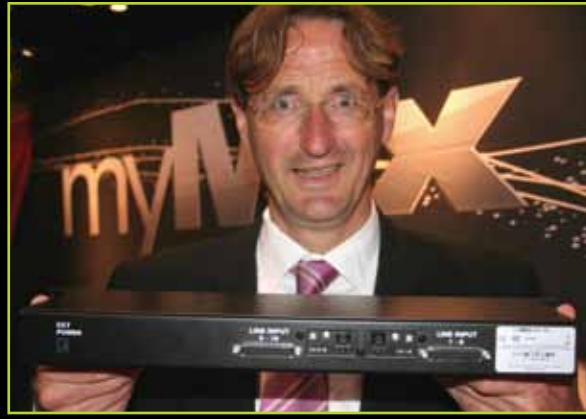
Movek's Mathias von Heydekampf with myMix IEX 16L-A , a 16-channel input expander that now has two 8-channel digital inputs on dual ADAT Lightpipe connectors, allowing 16 channels in 24-bit/48kHz to be imported into a myMix system.
